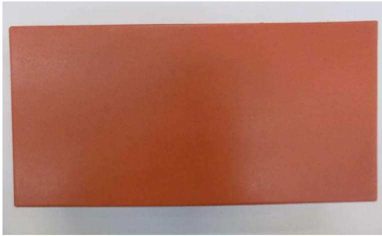
Figure 9 – Close-Up of the Unit after Application and Removal of Staining Media
