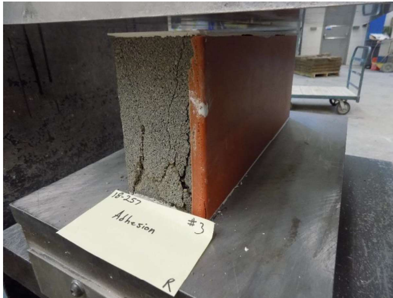
Figure 6 – Post Compression Testing Unit Face
