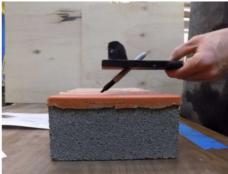
Figure 4 – Application of Magic Marker Spotting Media
