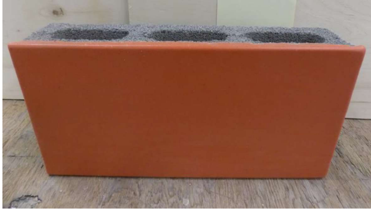
Figure 1 – As-received Concrete Masonry Unit with “Spectra Glaze II” Material
